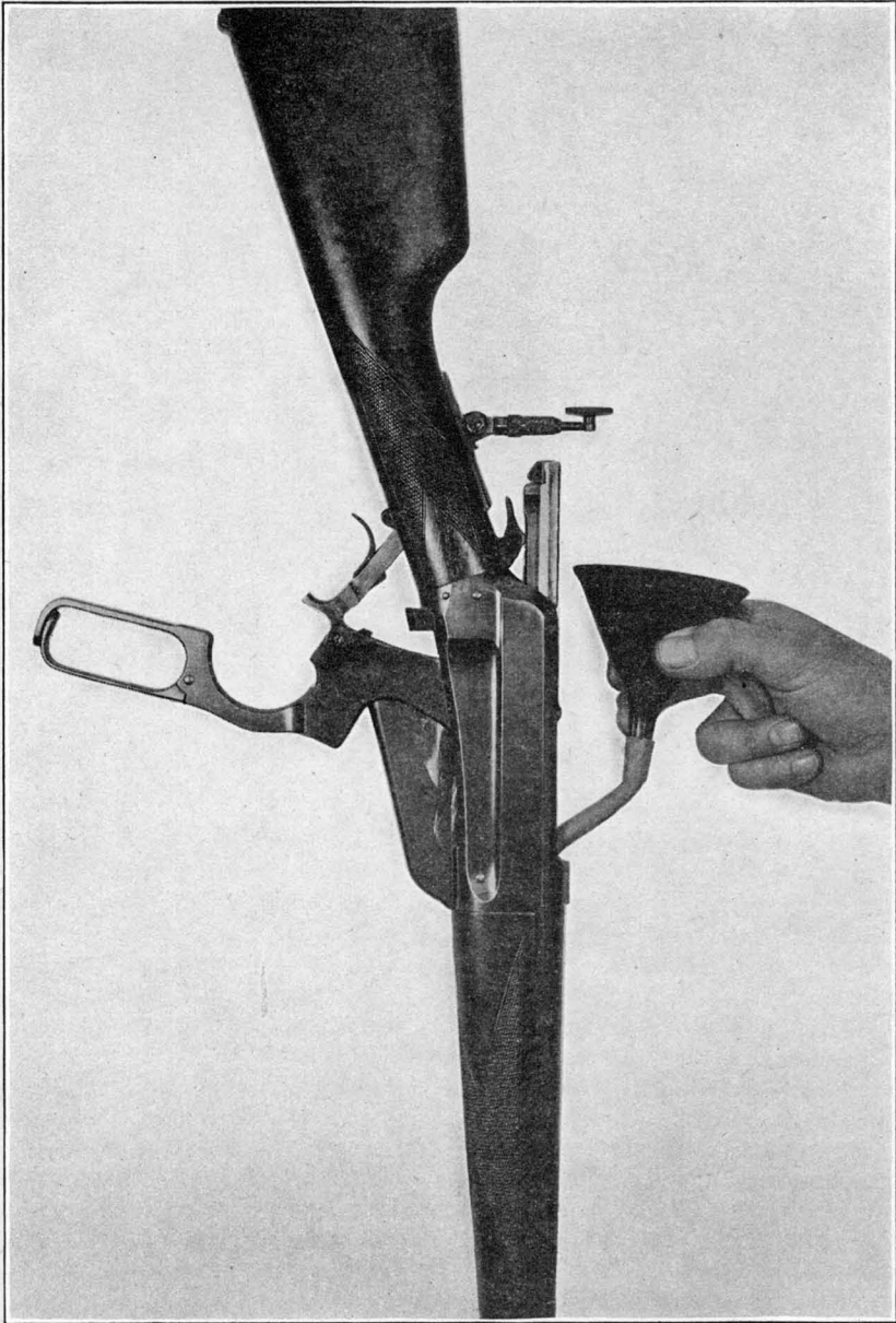
Figure 10. Funnel and tube for water cleaning
